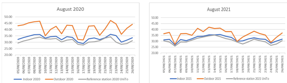
Figure 23. Maximum daily temperature inside and outside the shelter as measured in August 2020 and August 2021, compared with the temperature measured by a reference station (image @ CNR).
