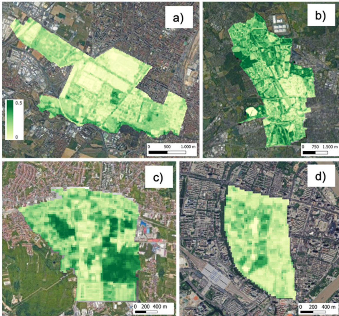
Figure 5. NDVI calculated at the Living Lab district level for Turin (a), Dortmund (b), Zagreb (c) and Ningbo (d) in 2019.
